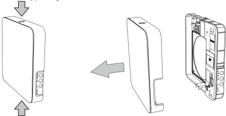
5 - Install the electronic part with the supplied screws and disassemble the right cover plate.
