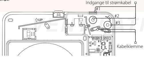
If input #1 on the top of the unit is used, the provided template in the center of the mounting template should be used to mark the notch. Drill out the notch so that the cover can be easily mounted and removed from the unit.
